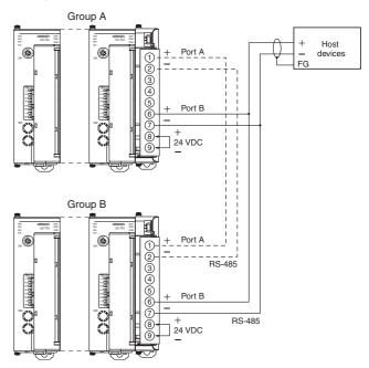
Note: Wire the dotted line when settings for all distributed Units are being made from one port A connector.If the dotted lines are not wired, make the settings for group A using the port A connector for group A and make the settings for group B using the port A connector for group B.
