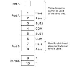
To connect to the G3ZA, separately purchase a G3ZA Connecting Cable (EJ1C-CBLA050) and connect it to the G3ZA connection port (CN1) on the EJ1. Note: 1. To connect to a computer using the port A connector, use a separately sold E58-CIFQ1 USB-Serial Conversion Cable. The Temperature Controller can be connected to a computer using USB. 2.
