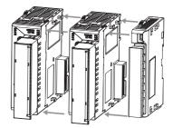
Note: 1. Do not connect the End Unit directly to an HFU.
