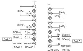
RS-485 for port C and RS-232C can be switched A separate EJ1 model must be used for RS-422 communications
