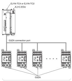
Up to 8 G3ZA Power Controllers can be connected to one Basic Unit.
