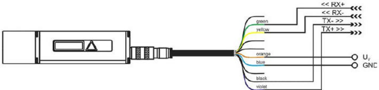
Figure 16 RS422 wiring diagram
