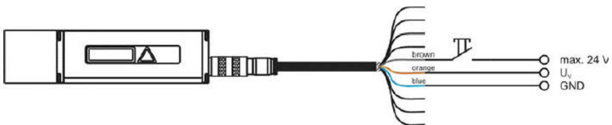
Figure 21 Wiring diagram of trigger input
