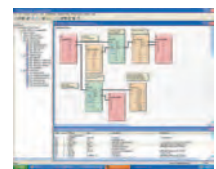
CX-Process Tool (Loop Controller Programming Software) ● Loop Controller program creation (function block method) ● CSV tag file output
